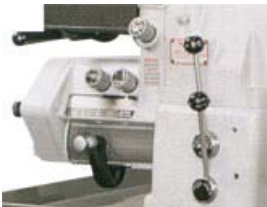
Dual range Inch/Metric quick change gearbox.
