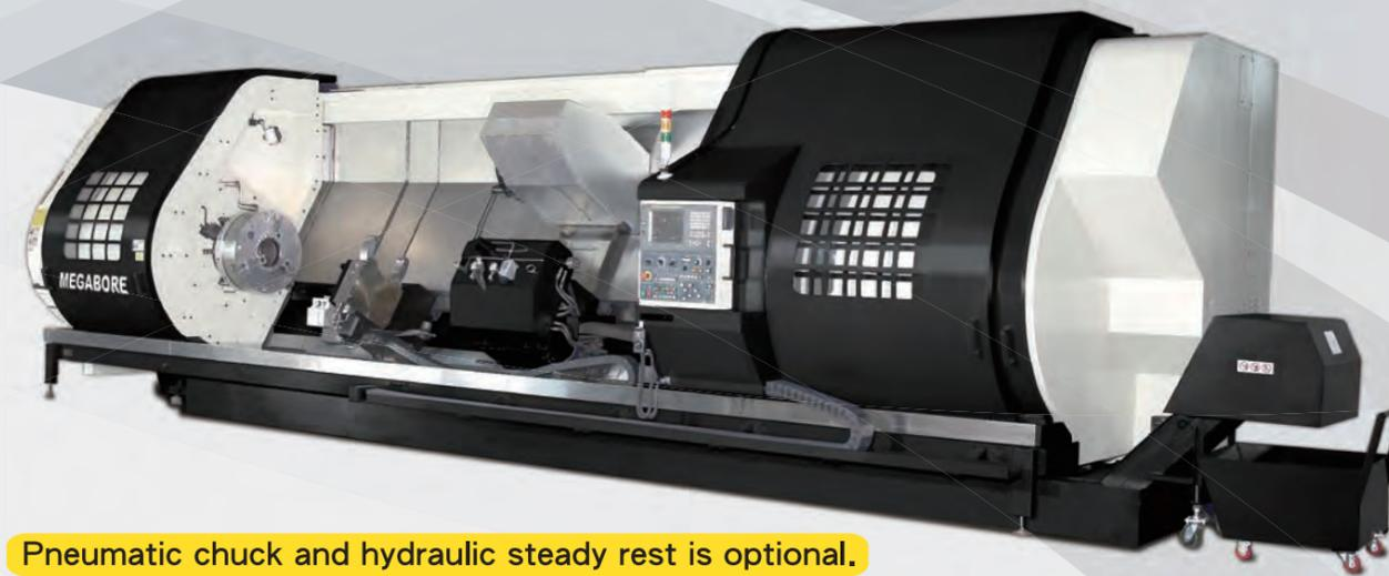
Pneumatic chuck and hydraulic steady rest is optional.
