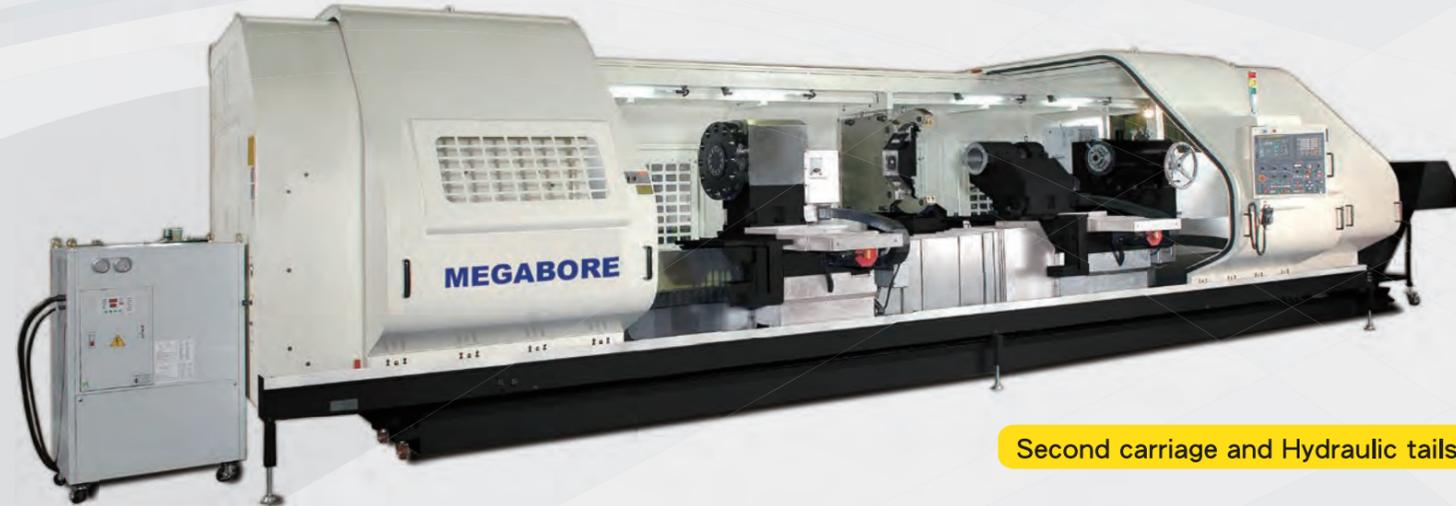
Second carriage and Hydraulic tailstock is optional.
